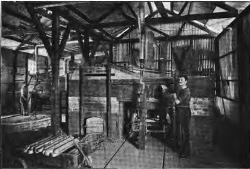
FIG. 66.—CUPELLATION FURNACES, GOLDEN HORSE-SHOE WORKS.
