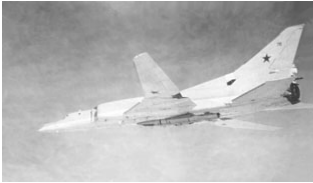
Tu-22M Backfire is a medium range bomber, capable of carrying gravity bombs and cruise missiles. Unilateral Soviet declaration of 31 July 1991, limited total holdings to 300 planes, of which 200 could be assigned to naval aviation. In this photo the Backfire is armed with the AS-4 Kitchen long-range, air-launched, cruise missile, capable of carrying either a 1,000-kilogram conventional or 350-kiloton nuclear warhead.
